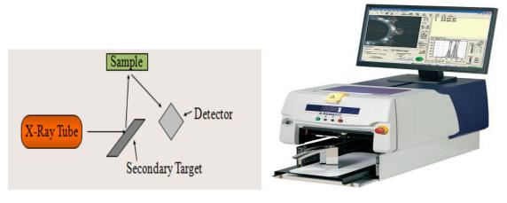
X-strata-920 XRF device the device analyze up to three layers, top layer Au (gold coating thickness), second layer Ag (silver coating thickness), the third layer Cu (copper coating thickness). It may analysis more layers such as palladium, platinum, nickel; if we have the identity standard disc of the required measurement.
